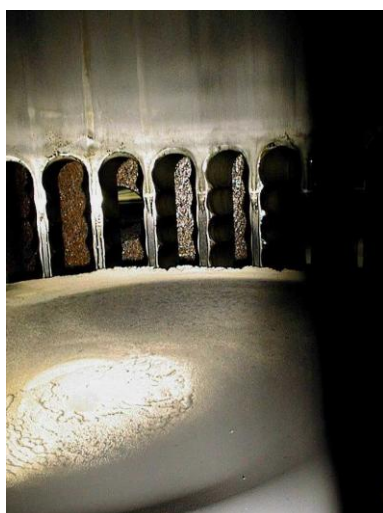
Excessive calcium deposits on piston
