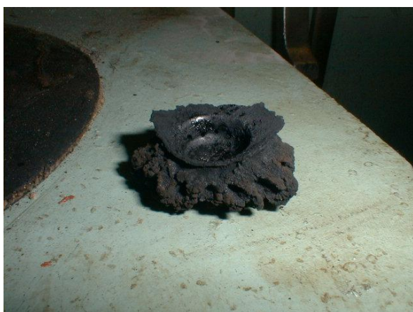
Excessive carbon deposits on injector nozzle tip often referred to as
