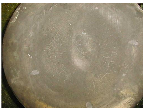
Piston crown corrosion/erosion
