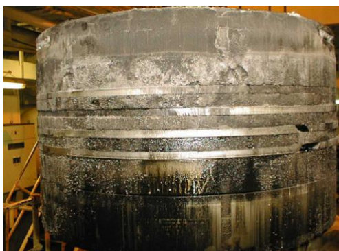
Piston fouling, ring seizure and loss of tension
