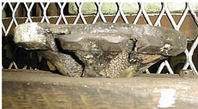
Damaged exhaust valves caused by hot corrosion
